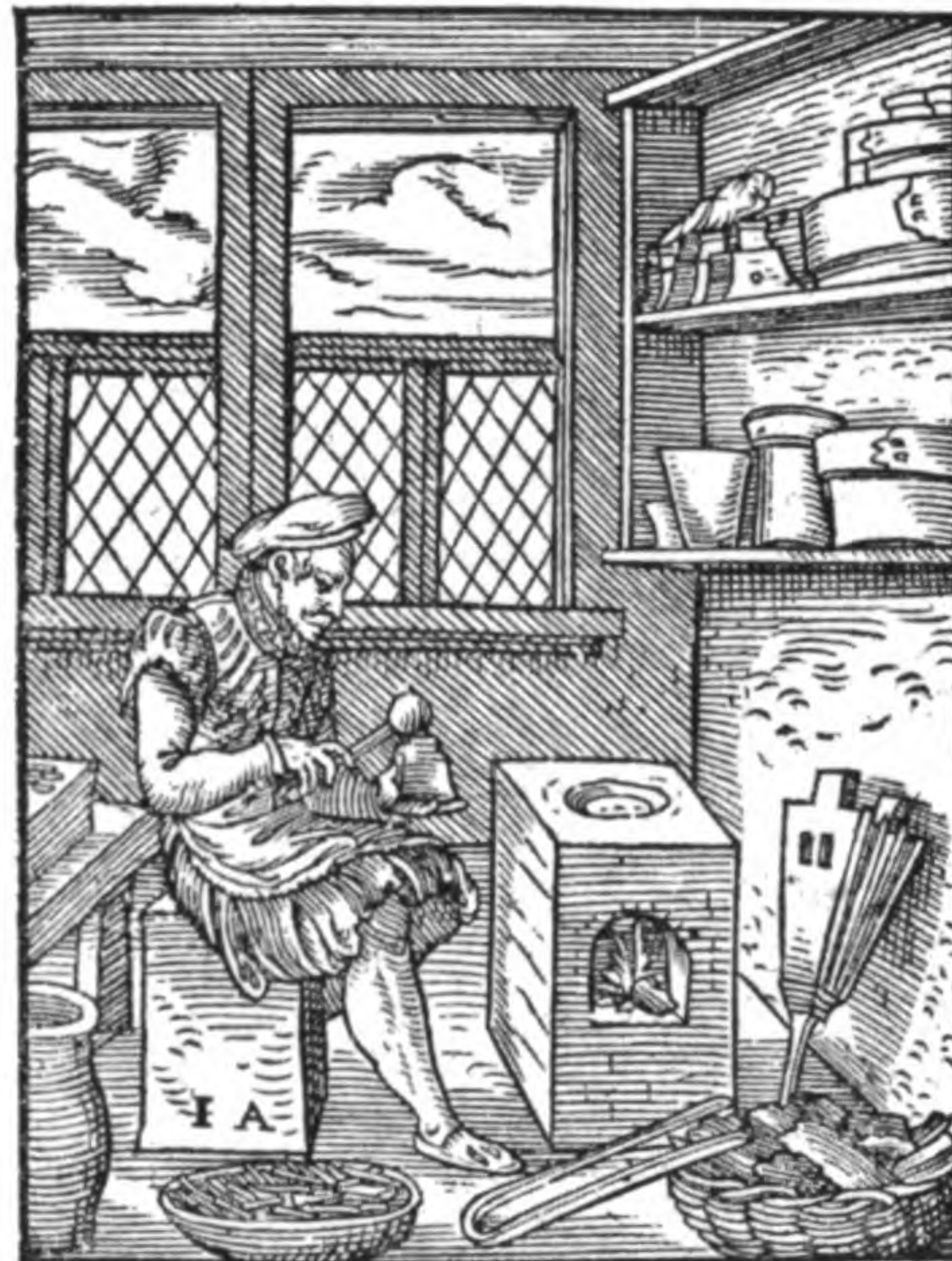
Earliest picture of typecasting from a wood cut by Jost Amman, published in 1568, in Frankfort-on-Main, by Sigismund Feyrabendt. The caster is pouring the metal into a mold. Extra molds on top shelf, at rear. Behind the caster a rubbing stone, on table, by which the bodies of the types were finished.
