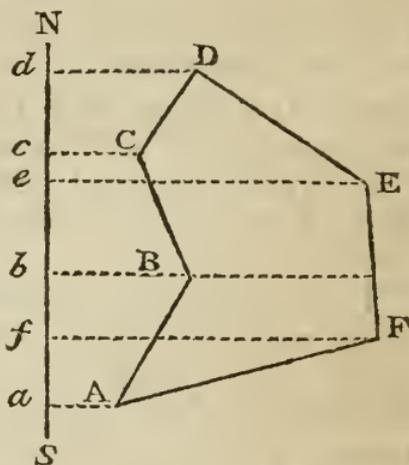
Then, I say, the difference between the sum of the products  $Aa + Bb \times a b$ ,  $Bb + Cc \times b c$ ,  $Cc + Dd \times c d$ ; and the sum of the products  $Dd + Ee \times d e$ ,  $Ee + Ff \times e f$ ,  $Ff + Aa \times f a$ ; will be double the area of  $ABCDEF A$ .
