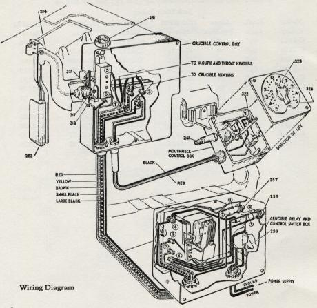
down the arcing effect of D.C. current. In installing the D.C. wiring, the polarity at the mouthpiece switch terminals must be as indicated at points 7 and 8 on the wiring diagram. If not connected in this manner, reverse the two wires at these points.
