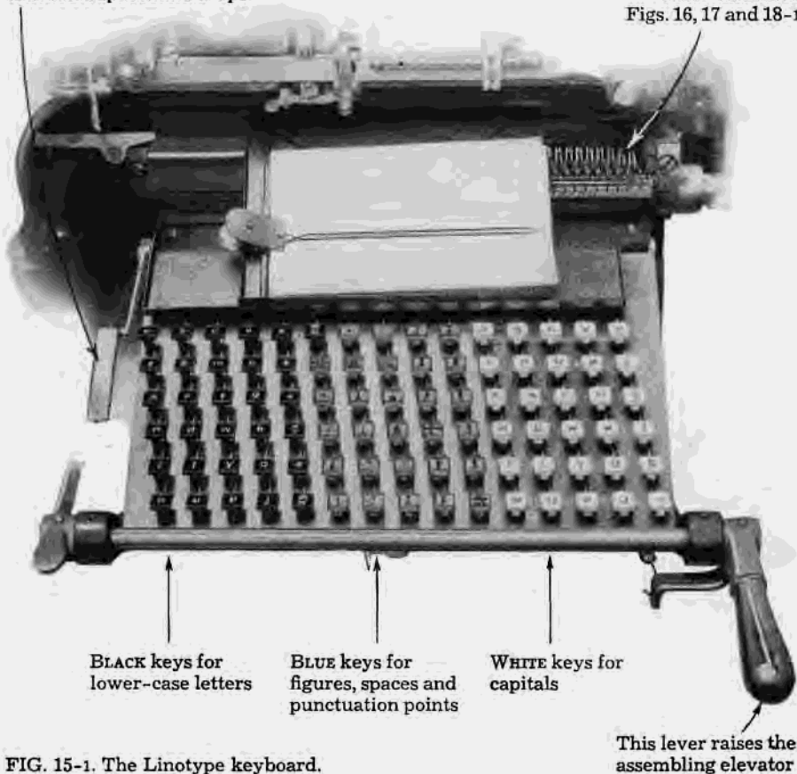
FIG. 15-1. The Linotype keyboard.
