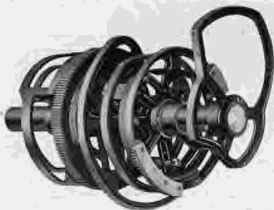
FIG. 3-1. The cams assembled on the shaft actuate and control most of the mechanical actions of the Linotype. A one-third horse-power motor drives the entire machine.
