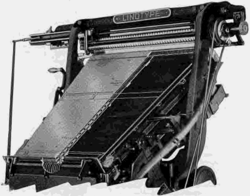
FIG. 6-1. Linotype matrices are stored in magazines, from which they are released as explained on page 9. In this illustration the upper magazine has been cut away longitudinally to show all matrices of one character in "channel" which retains them.
