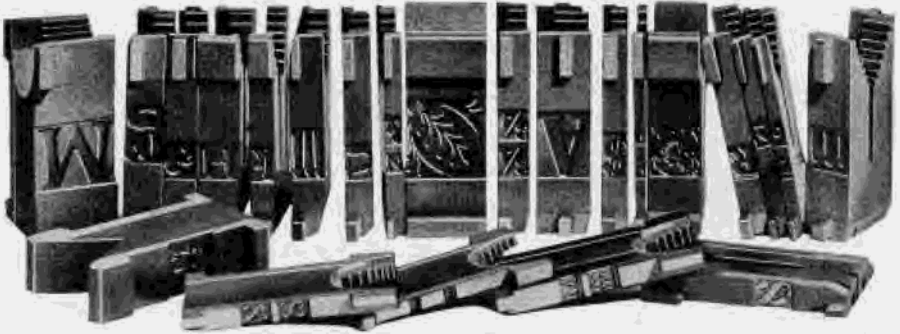
FIG. 5-1. A few matrices of a wide variety of characters commonly used in printing. They are made in sizes from 4 point to condensed 60 point.
