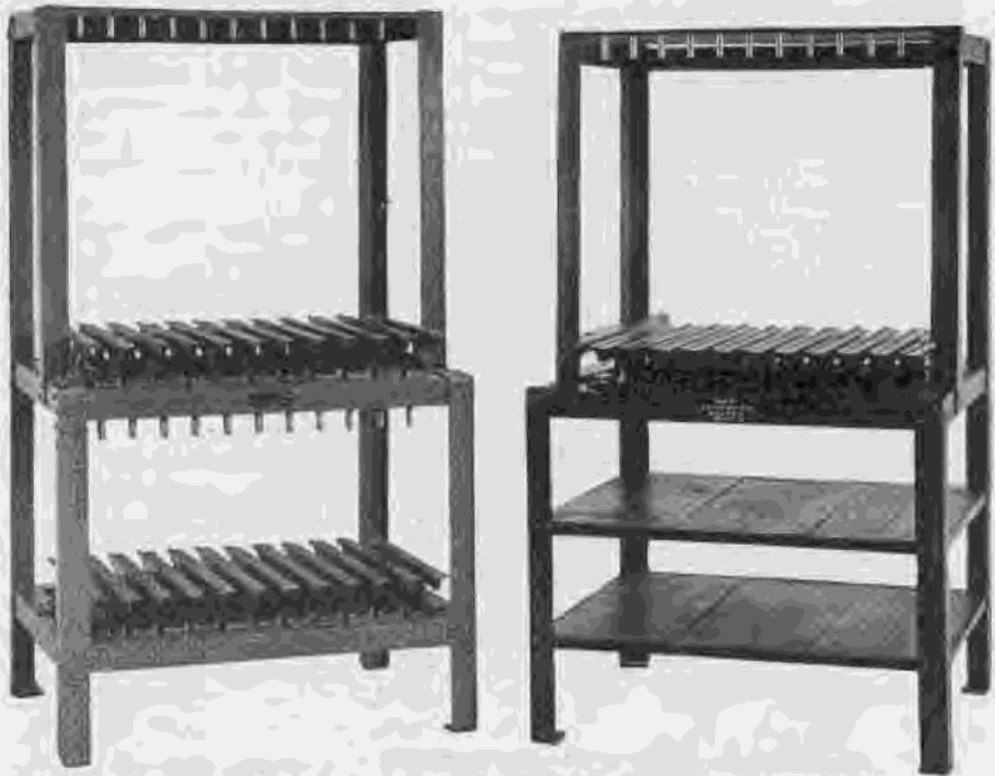
FIG. 60-1. Several styles of racks are available, for storage of various combinations of extra magazines, either full-length, split or auxiliary.
