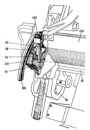
FIG. 12-26. View of channel frame and cam plates in operating position.
