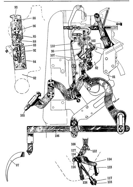
FIG. 11-26. Diagram of assembled "Two-in-One" mechanism for Model 32 Linotype, with channel entrance and distributor bar in 90-character operating position. Additional enlarged views show at upper left, the revolving block and fixed plate in locked position; and, at lower right, the safety device which operates in conjunction with the matrix guard.
