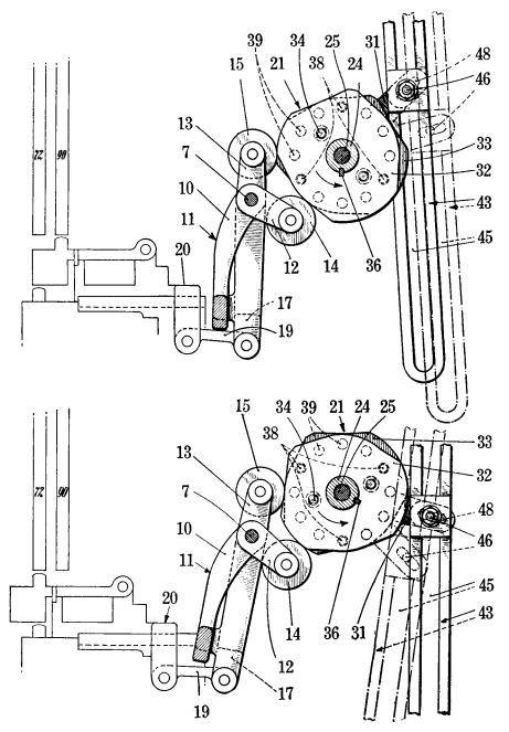
FIG. 5-26. The upper view represents a vertical section of the Channel Chooser showing the cam portion and keyboard rod lever slide in position to operate 90-character magazines. The lower view shows the keyboard rod lever slide in position to operate 72-character magazines.
