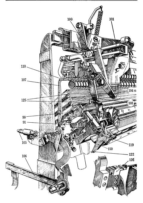
FIG. 10-26. Perspective view from rear of machine, with channel entrance bracket in phantom, showing channel entrance unit and distributor shifter levers in position to complete the change from 90-character operation to 72-character operation.
