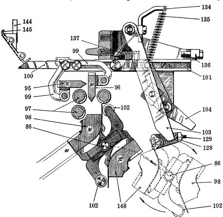
FIG. 13-26. Diagram of channel entrance unit and distributor bars in position for 90-character operation. The dotted outline of the channel entrance unit indicates its travel in effecting the change from 90- to 72-character operation.
