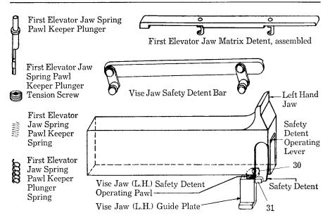
FIG. 7-32. View showing details of the vise jaw left-hand safety detent and first elevator jaw matrix detent.
