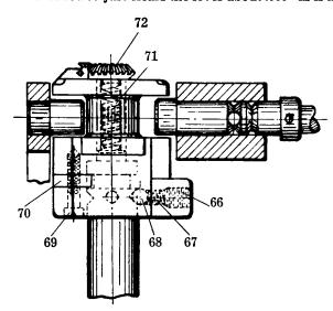
FIG. 15-32—Construction of vise jaw control rod latch with the operating studs engaged.
