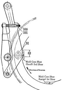
FIG. 18-32. View of the mold cam and driving gear when standing at right-hand side of machine, showing the mold cam roll and eccentric pin. The eccentric pin and roll are part of the solid type of mold cam lever and the eccentric pin is used to make the adjustment for the proper clearance between face of mold and matrices when justification takes place.
