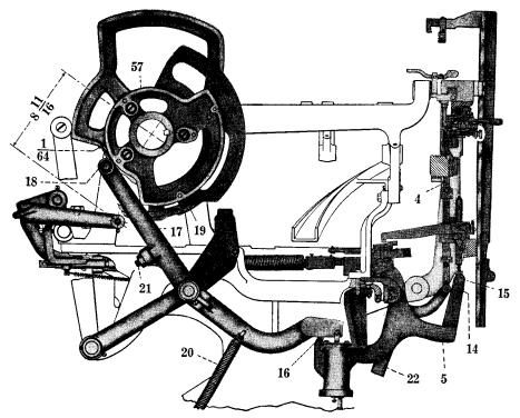
FIG. 4-32. Side view of the Self-Quadder mechanism.
