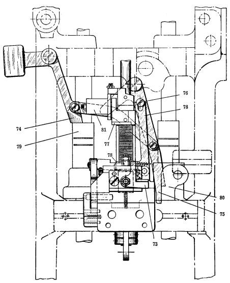
FIG. 16-32. View of the mechanism for controlling justification. The justification stops permit the spaceband driver to rise when machine is being used as "Regular" and prevents it from rising when Self-Quadder is in use.
