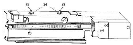
FIG. 5-32. View of the first elevator front jaw with the matrix detent in position to steady the last matrix of the line.
