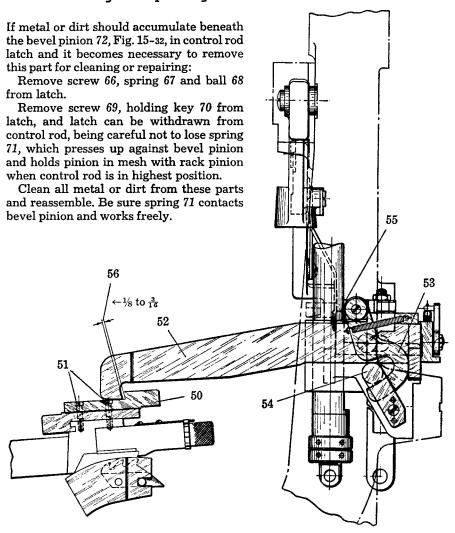
FIG. 12-32. View showing the mechanism for applying the extra pressure to the vise jaws after the toggle lock is in the locked position. This extra pressure against the line of matrices assures a tight line.
