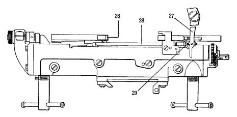
FIG. 6-32. View of the vise cap and vise jaws showing the vise jaw left-hand safety detent and the pump stop lever operating lever.
