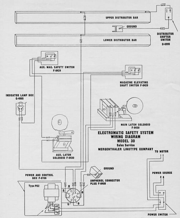
For 220 V. AG, connect 717 to term. 11; 716 and 719 to term. 12; 720 to term. 13 For 110 V. AG, connect 717 and 716 to term. 11; 719 and 720 to term. 13
