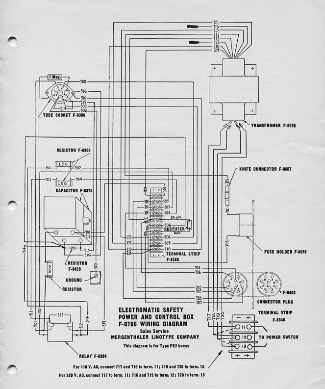
type fuse must be used. These can be ordered from the Mergenthaler Linotype Company or may be procured locally in an electrical supply shop. It is suggested that spares be kept on hand.
