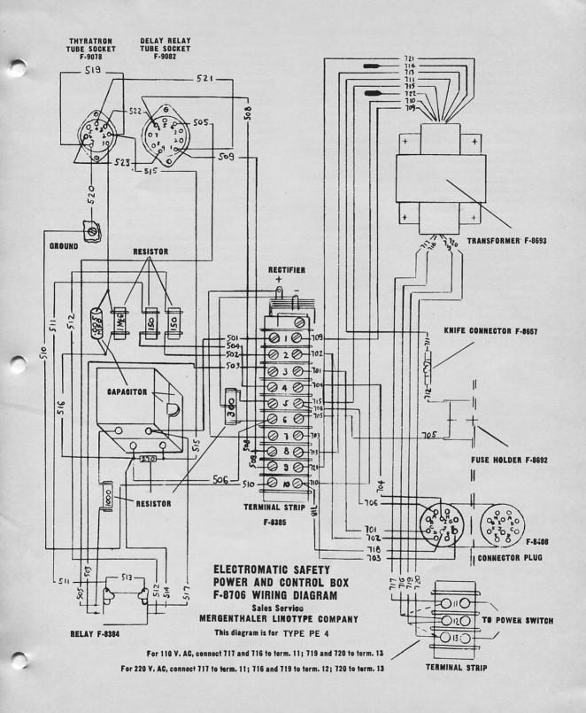
machine order. If it is necessary to change the voltage from 220 volt A.C. to 110 volt A.C., or vice-versa, the connections to the transformer must be changed as shown on the diagram. The transformer primary coils are connected in series for 220 volt and in parallel for 110 volt operation.
