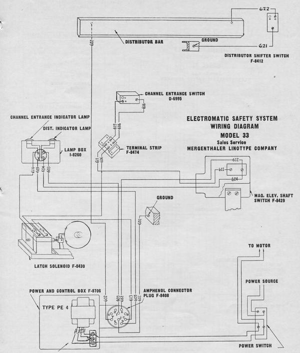
For 220 V. AC, connect 717 to term. 11; 716 and 719 to term. 12; 720 to term. 13 For 110 V. AC, connect 717 and 716 to term. 11; 719 and 720 to term. 13
