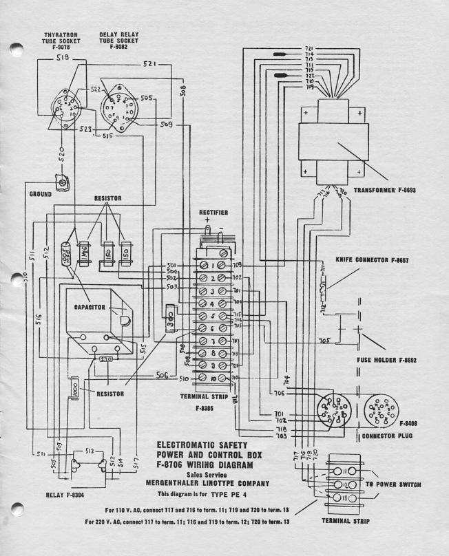
The Thyratron tube and the Amperite delay relay tube located in the power and control box F-8706, are standard tubes carried by most radio supply dealers. However, it is suggested that these tubes be ordered from the Mergenthaler Linotype Company where they are pretested to assure correct operating characteristics. It is also suggested that spare tubes be kept on hand.
