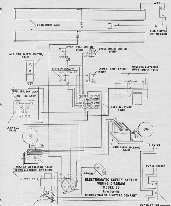
For 220 V. AC, connect 717 to term. 11; 716 and 719 to term. 12; 720 to term. 13 For 110 V. AC, connect 717 and 716 to term. 11; 719 and 720 to term. 13
