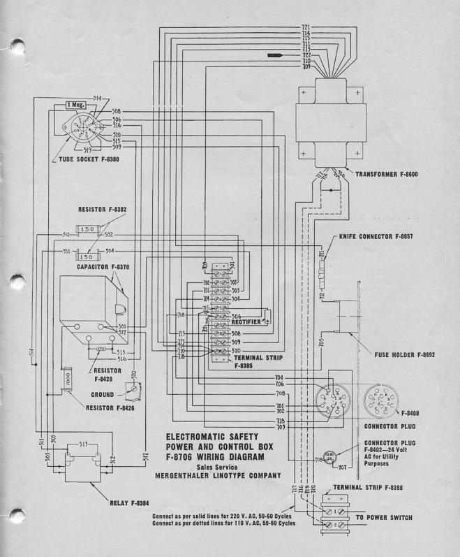
trol box F-8706 by pulling out the amphenol connector plug F-8408.
