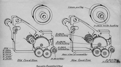
D-3304 Model 5B-8B D-3499 Model 8c-14B.5.k-/4C-21B-22B.5.k D-5019 Model 8BB-25B-29(2)(90)-29(4)(90)-31(4)(90)
