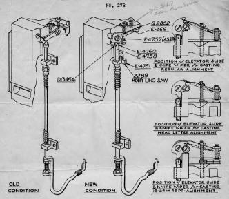
MEANS TO AUTOMATICALLY REGULATE THE STROKE OF THE KNIFE WIPER WHEN CHANGING THE CASTING POSITION
