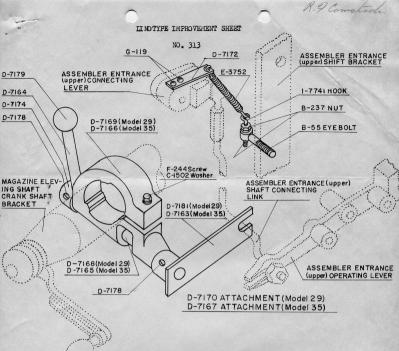
MANUALLY OPERATED OSCILLATING FRONT SHIFT
