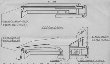
First Elevator Jow Line Stop Transfer Rod Guard (Assembled)(New) <u>E-4456 (30-36Em)</u> E-4459 (42Em)
