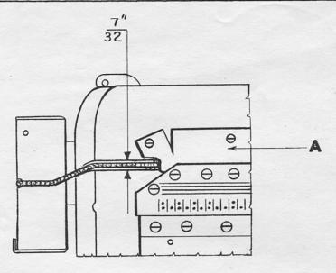
Remove guard A and place mouthpiece probe in its groove in back of mouthpiece. Do not pack with asbestos since this may affect control of mouthpiece temperature. If a Comet type electric pot is used, insert probe in hole in front of mouthpiece heater. If it is difficult to put in the probe from the left of the mouth heater, insert lead wires in the hole at right of heater and pull the probe through from right to left.
