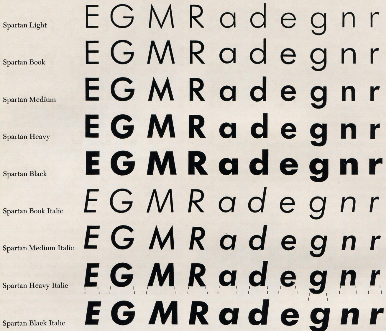
FIG. 7—Typical letter forms in the five weights of the Spartan Family, reproduced from their matrix patterns in approximately 48-point size, permit study of their details. The fine marks just below the Heavy Italic compare the set widths of that face with the set widths of the Black Italic in the line below. The set widths are fairly constant for the lighter weights, as compared with the added width needed to preserve the family traits in design for the Spartan Black.
