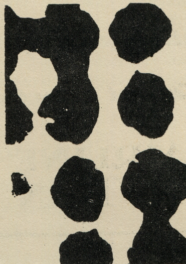
2. Dots Flatten and Fill on Newsprint—Same section proofed on newsprint.
