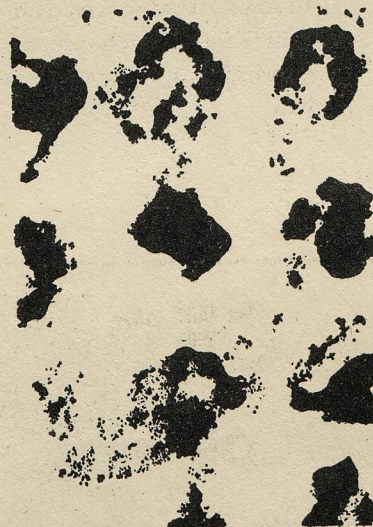
4. The Reproduction in the Newspaper—The identical halftone screen dots as they actually appeared in the newspaper. NOTE: This example was taken from a well-printed halftone.
