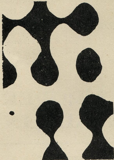
1. The Halftone Dots as They Actually are—Proof carefully pulled on coated stock and enlarged.
