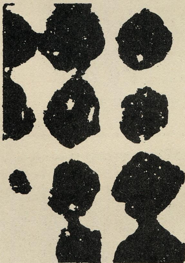
3. Stereotyping Doesn't Help—The dots lose some of their solidity when the plate is stereotyped.
