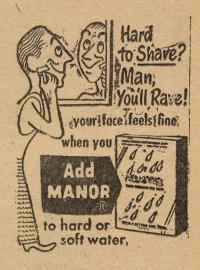
This is the result of a mat made from a shallow pattern plate. Note filling in around type and illustration at top of advertisement.
