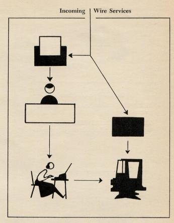
REPERFORATOR receives and punches wire copy as received, edited for group of papers, TTS punched and sent out over circuit wire.
