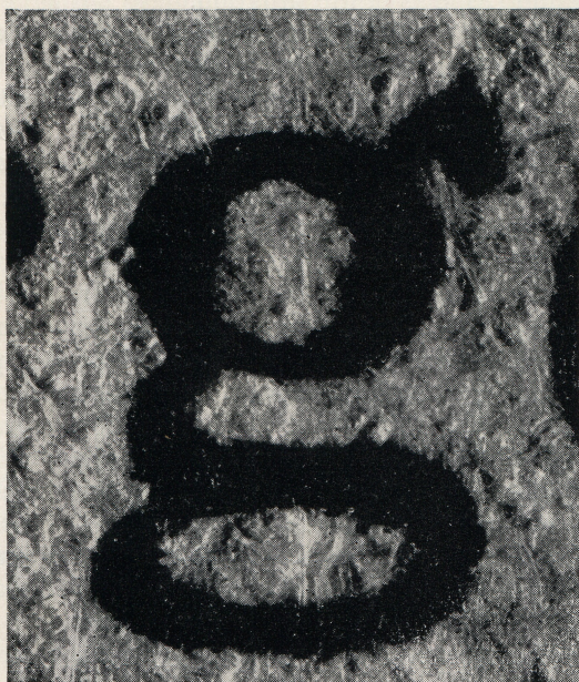
FIG. 1—Newsprint enlarged about twenty-five diameters, carrying an impression of Corona.
