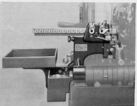
Square halftone, 133 line, no line. Made from retouched photographs. The separate halftone negatives were stripped together and the white lines between the views were cut in the plate.
