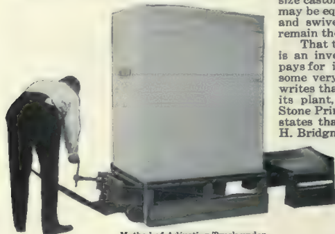
Method of Adjusting Truck under Loaded Platform
