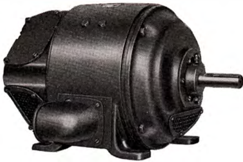
Dripproof, fully protected Type B or CD motors. Note solid covers on all top ventilating openings for dripproof construction and perforated protective covers for all other openings
