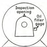
External plan view of sleeve-bearing housing
