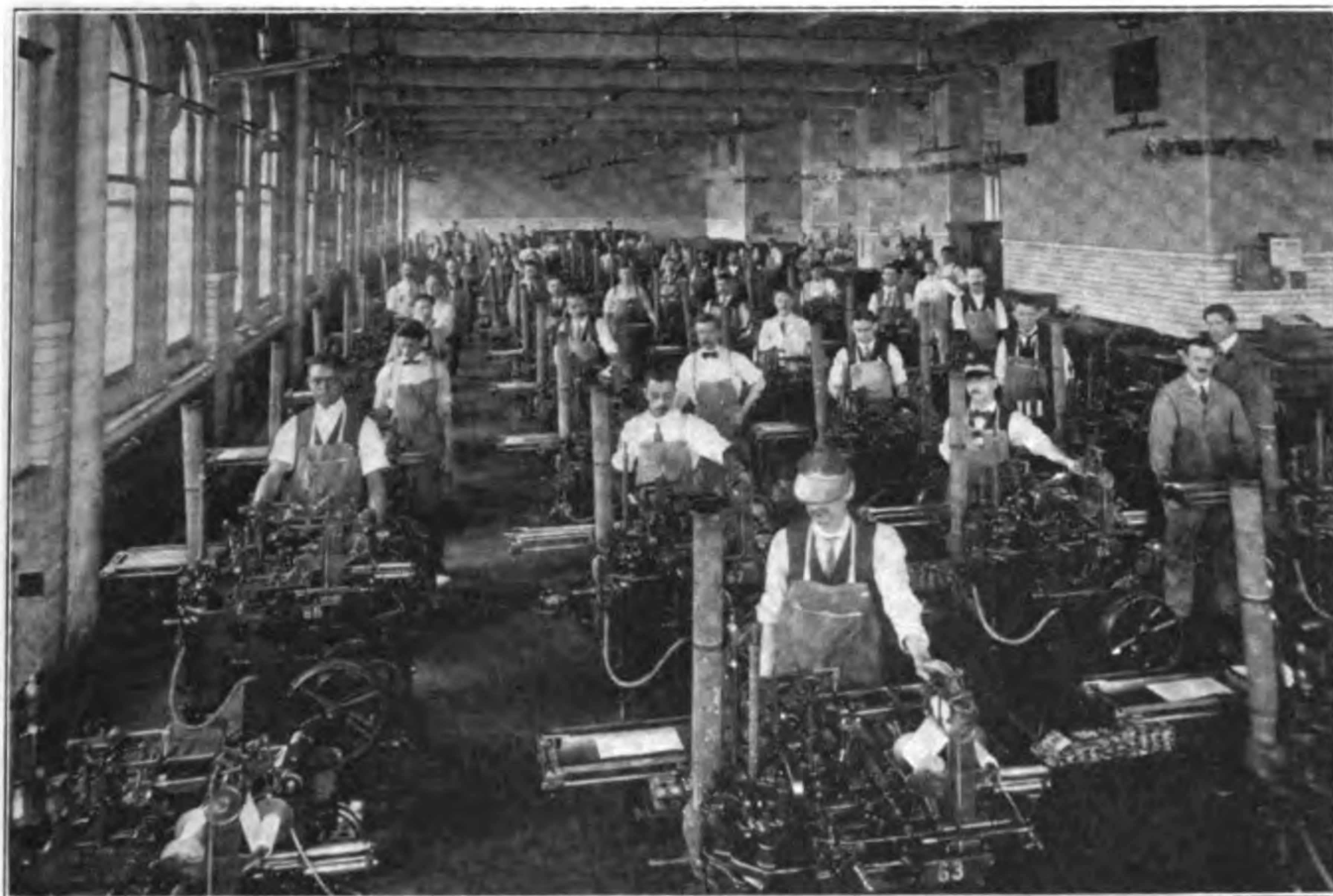
A view of the largest battery of composing machines in the world. The Government Printing Office at Washington, D. C., operates 126 Casting Machines
