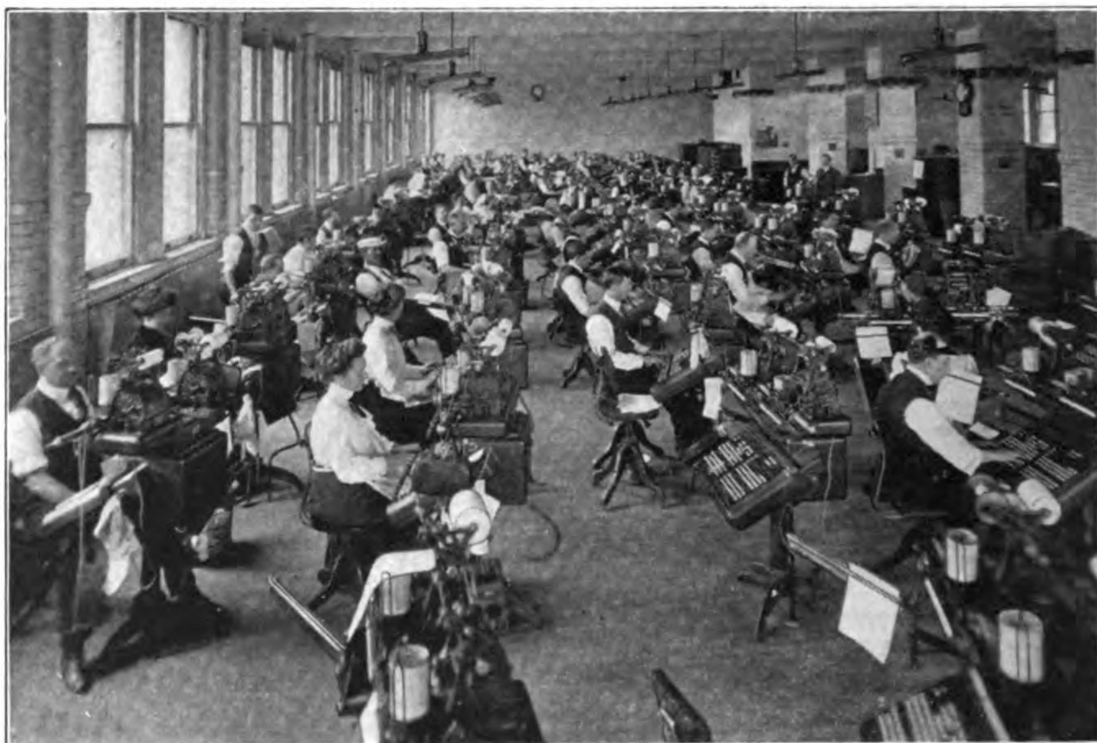
A view of the largest battery of composing machines in the world. The Government Printing Office at Washington, D. C., operates 100 Monotype Keyboards
