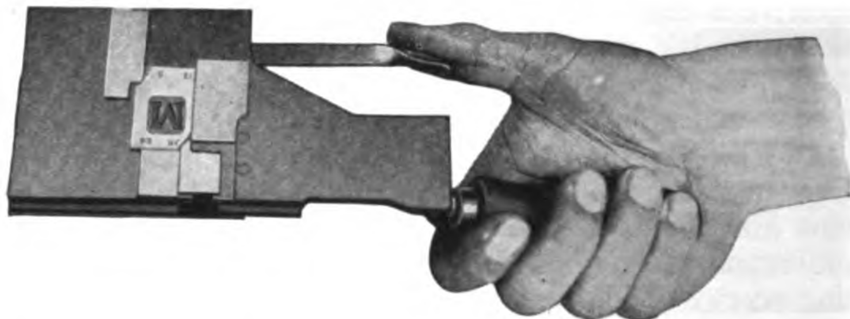
FIGURE 1 SORTS MATRIX HOLDER: Holds Sorts Matrices, one at a time, for casting type for the case. To change a matrix, press the Latch with the thumb as shown and pull out the Slide (Fig. 2); the Holder itself remains in the machine.
