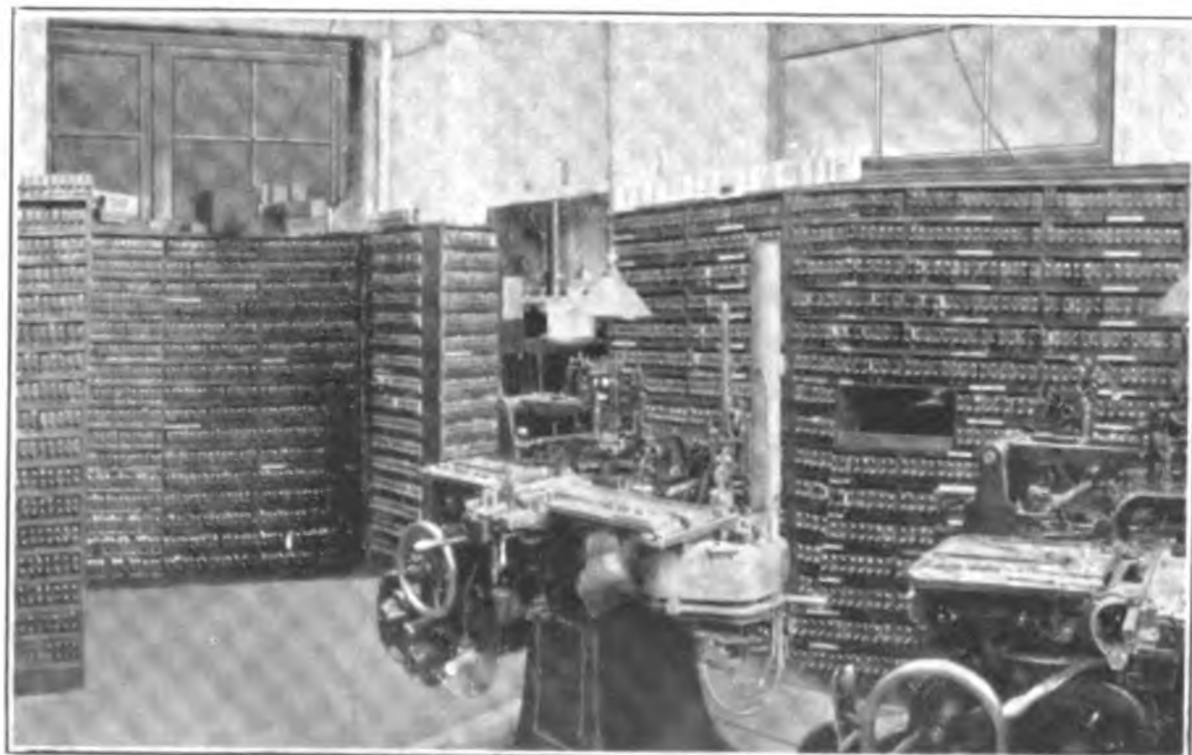
Type Casting and Storage Section of the Philadelphia Record, showing Monotype Type-&-Rule Casters and Storage Cabinets and how large storage capacity was obtained by following contour of walls.
