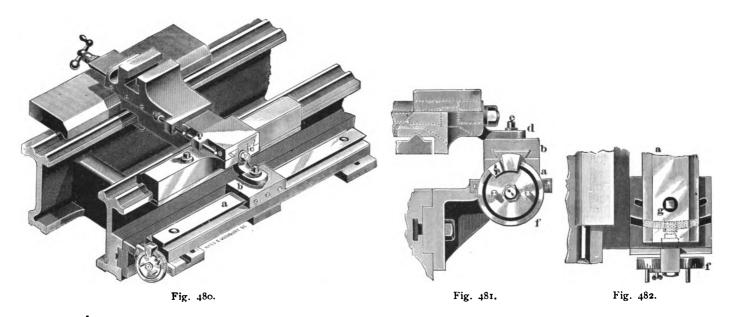
the support 8 moves in the dovetail channel of the plate 7, it acts as a bearing for the plate 7, and retains said plate in proper position in alignment with the bed to secure perfect action of the parts. The bar 2 is adjustably connected with the tool-holder to vary the position of the same for different work.
