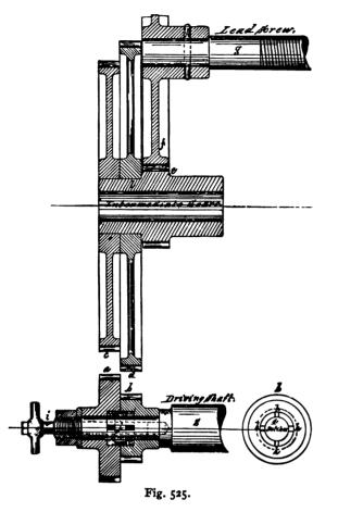
by p' in the end view; upon this pivot operates the piece D, having the handle d. In D are two cam grooves a a; two pins n, which are fast in the two half-nuts N N', pass through slots c c in B, and into the cam grooves a a respectively.
