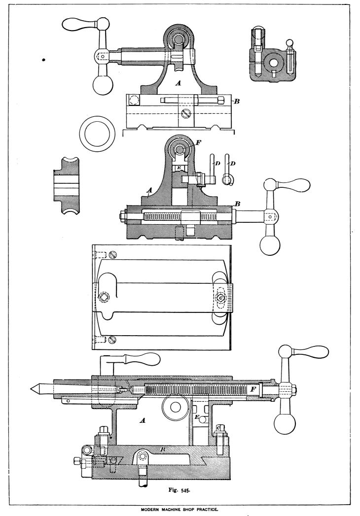
Manufacturing Company of New Haven, Connecticut. The compound rest is here provided with automatic feed so that it may be set at an angle to bore tapers with a uniform feed. The tailstock is provided with a bracket, carrying a pinion in gear with the hand-feed rack, so as to move the tailstock along the bed by means of the pinion. The feed screw is splined to give an independent feed, and the swing frame is operated by a worm as shown.
