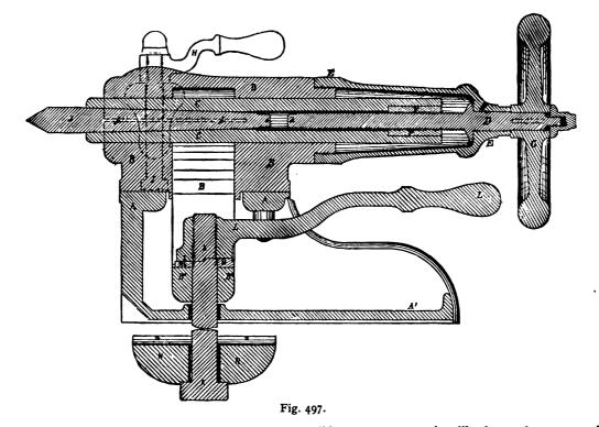
rotating the handle L in the necessary direction lifts K and causes N to rise, and grip the shears beneath, while the pressure of M on B" causes B to grip A and the latter to grip the raised Vs on the shears. If L be rotated in the opposite direction it will cause N to fall, leaving A free to slide along the shears. To prevent N from partly rotating when free, its ends are shaped to fit loosely between the shears as shown at n.
