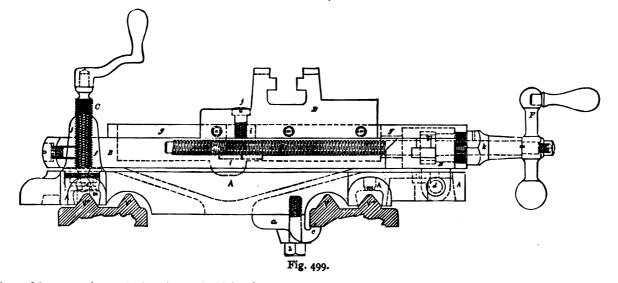
A two lugs f, between the vertical surfaces of which B is a close working fit. The upper surface of B is provided with a V-slide way g, to which is fitted the tool rest D (the construction being more clearly shown in Fig. 500).
