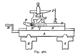
turned by the tool whenever the pivot D was on the handle H side of the line of ce. tres. To steady C it may be provided with a circular dovetail, as shown at the end I, provision being made (by set screw or otherwise) for locking C in a fixed position when using the rest for other than spherical work.
