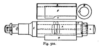
radial face, and the nut W affords the other radial face, preventing end motion to x without moving P endwise. If x be rotated its thread at x' causes it to move laterally, carrying P with it, and P being fast to P' also moves it laterally. P' is maintained from end motion by a groove at O' in which the end of a screw a projects, a screwing through W and into the groove O'.
