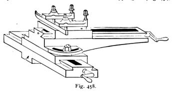
are on the right-hand side, as in that figure, there is considerable strain on the screws when a boring tool is used to stand far out, as for boring deep holes. On the other hand, however, the screws can be readily got at in this position, and may therefore be screwed up tightly to lock up the upper slider firmly to the cross slide, which will be a greater advantage in boring and also in facing operations. But the screws must not, in this case, have simple saw slot heads, such as shown on a
