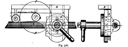
suppose d be raised, then the grooves a a would force their respective pins n up the slots c, and these pins n being each fast to a half of the nut, the two half-nuts would be opened clear of
