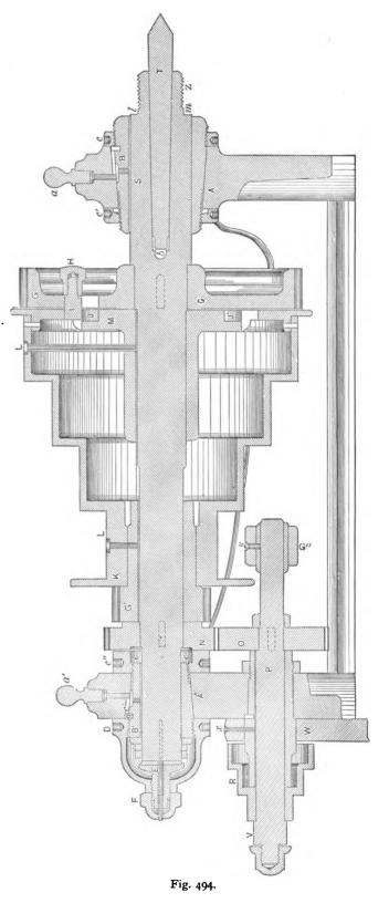
are then screwed up, withdrawing B and B' respectively, and leaving the journal fit too easy. C' is then screwed up until B is closed upon the spindle sufficiently that the belt being loose on the cone pulley, the latter moved by the hand placed upon the smallest step of the cone can just detect that there is contact between the bore of B and the spindle, then, while still moving the
