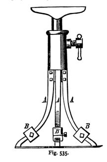
The distinguishing feature of this lathe is that the tailstock spindle is made square, to better enable it to bear the strain due to carrying cutting tools in place of the dead centre; and by means
