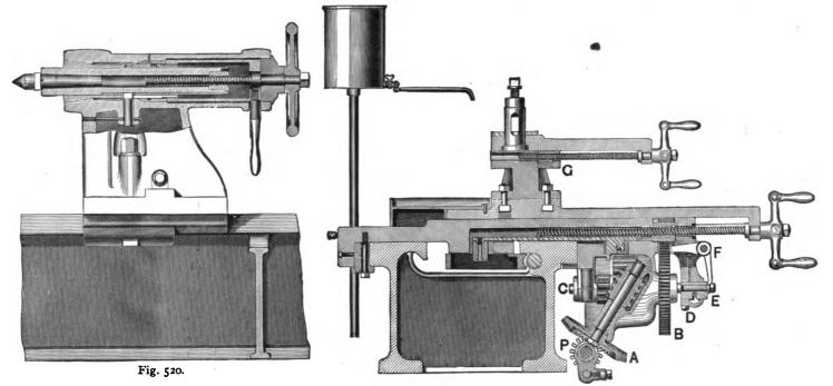
spur gear referred to is fast) is pulled endways outwards from the lathe bed, its front annular clutch engages with the clutch that sets the cross-feed gear B in motion, and B engages with a pinion which forms the nut of the cross-feed screw.
