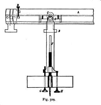
holes the slide rest must either be a compound one or a taper turning former or attachment must be employed.
