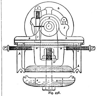
farther into A, the end of P' will meet the surface of B', causing B' to move over, and the centre of the dead centre J (which is the axis of rotation of the work at that end) will be nearer to the point of the cutting tool. Or suppose the work requires to be turned a taper having its largest diameter at the end running on the dead centre, then P' would be unscrewed and P screwed farther into A, carrying B farther towards the back of the lathe.
