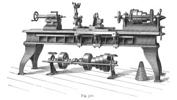
compound slide rest, thus increasing the capacity of the lathe not having a simple or single rest.
